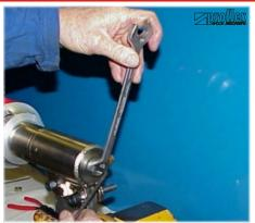
Replace the bottom securing nut and tighten firmly. Raise the spring platform to its original fitted spring length position.
