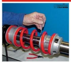
The four long bolts, already replaced, can now be fixed to the outer casing NOT TO TIGHT
