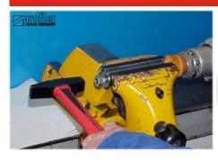
Replace the bottom nut by 5 turns. Using the open jaws of the vice, gently strike the nut to loosen the "fitted" washer. DO NOT TIGHTEN the vice against the rod.
