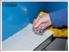
Remove the rubber 'O' ring from the end of the rod using the small screwdriver.
