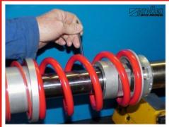
Using the "allen key" unscrew the four long bolts from the top bearing holder.
