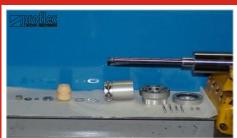
Remove the bumpstop, circlip and washer.
