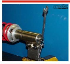
Hold the piston rod with the "allen key". Now remove the 19.0 mm nut.
