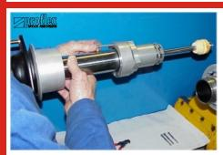
Insert the four long bolts into the top bearing holder.
