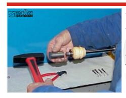
After cleaning you must grease all the parts and reassemble.
