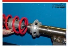
Holding the unit as shown, withdraw the insert and spring from the outer casing.
