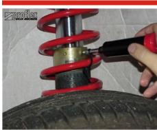
NOTE : Replenish the grease in the top seal housing in this way every 4 Special stages. This may vary depending on the length of stage and surface conditions.
