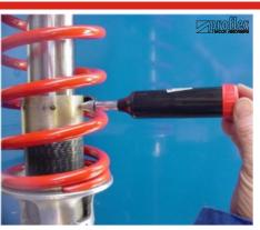
Apply grease through this hole using the grease gun supplied. Replace the grub screw. The shockabsorber is now ready for fitting to the vehicle.
