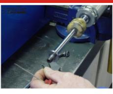
Remove the rubber 'O' ring from the end of the rod using the small screwdriver.
