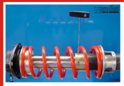
Raise the spring platform to its original fitted spring length position.
