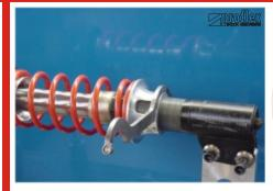
Measure the fitted length of the spring before relieving the spring tension, using the special tool provided to lower the spring platform.
