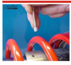
Release/remove the small grub screw in the top seal housing.
