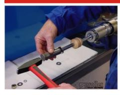
Reassemble the parts. Re-fit the end washer using the special drift provided.
