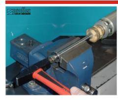
Replace the bottom nut by 5 turns. Using the open jaws of the vice, gently strike the nut to loosen the "fitted" washer. DO NOT TIGHTEN the vice against the rod.
