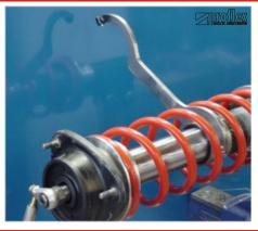
Using the special tool provided, unscrew the top seal housing and disengage the threads.
