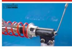
Re-fit the top seal housing and tighten firmly. Replace the bottom securing nut and tighten firmly.
