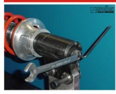
Hold the piston rod with the "allen key". Now remove the 19.0 mm nut.
