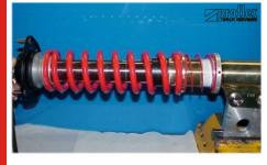
The spring and insert assembly can now be refitted to the outer casing.
