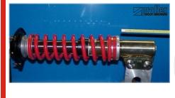
Measure the fitted length of the spring before relieving the spring tension, using the special tool provided to lower the spring platform.
