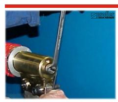
Replace the bottom securing nut and tighten firmly.
