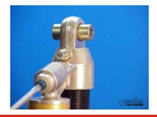
Use a screwdriver for adjustment of low speed compression damping Moving the adjusters in a clockwise direction "increases" the amount of damping, conversely moving in an anticlockwise direction "reduces" the amount of damping
