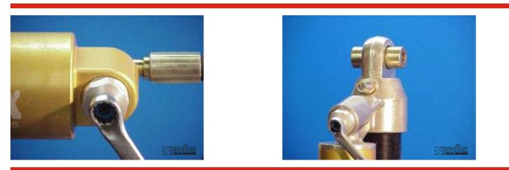
Use a 10.0 mm spanner for adjustment of high speed compression damping. DO NOT hold <u>low speed</u> adjuster whilst making high speed adjustments. Again move in clockwise direction to "increase" damping, and moving in an anticlockwise direction "reduces" the amount of damping
